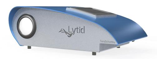
The TeraSchotty is a low frequency THz source based on state-of-the-art Schottky diodes multipliers chains. Available at 150 GHz, 300GHz and 600GHz center frequency with tens of mW of average output power, TeraSchottky provides the largest tunability on the market for multiplier based sources with >12% of center frequency. TeraSchottky is fully integrated, plug and play system and controlled with a capacitive touchscreen for the best user
