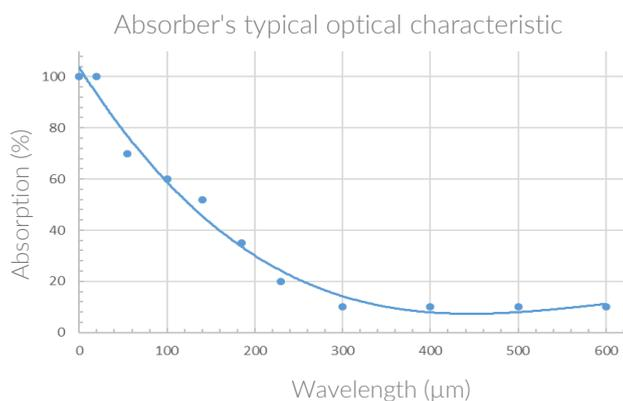
Figure 1 Absorption vs frequency of black coating
