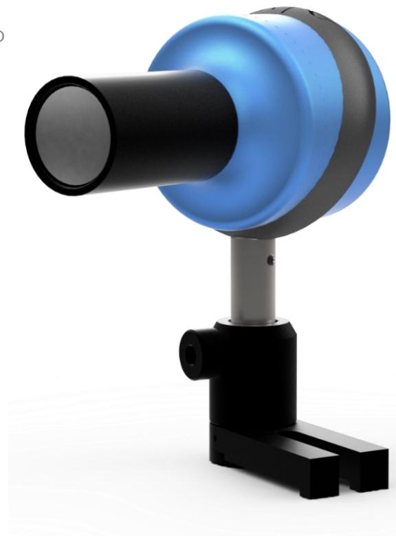
The TeraPyro sensor is a compact and highly sensitive device, based on the combination of a high-quality absorbing black coating, paired with a LiTaO<sub>3</sub> pyroelectric crystal. The broad absorption range of the coating allows the use of this sensor over a large spectral range (from 0.1 to 30 THz). The high sensitivity and low NEP offer no compromise on performances. The integrated, pre-aligned, high quality THz optics based on AR coated Si-lenses ensures
